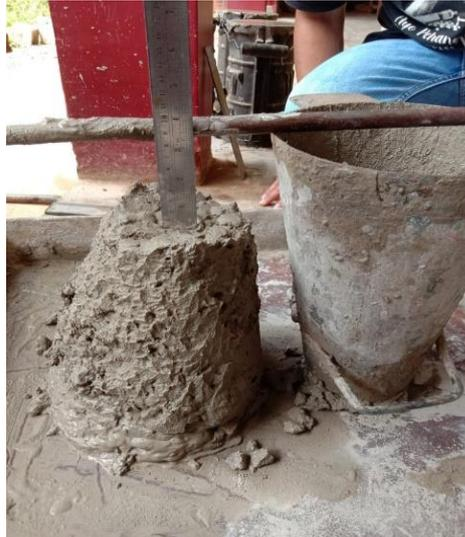
Gambar 6. Uji Slump Beton Segar
