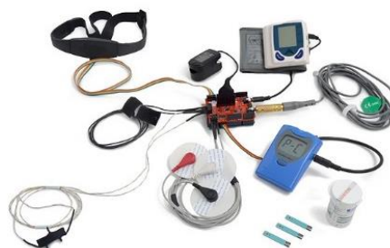
Figure 2. E-Health Sensor Platform V2.0
