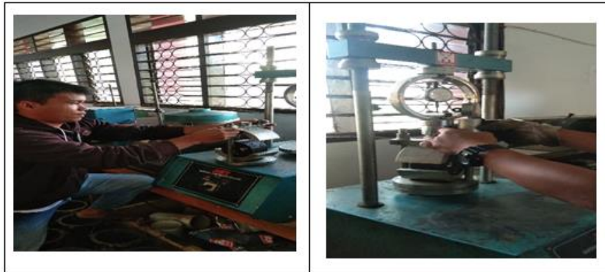
Figure 2. Marshall conventional test of AC-BC mixture
