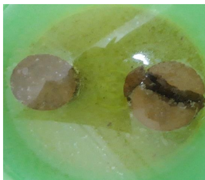
Figure 13. Physical appearance of specimen curing sulfuric acid ( H_2SO_4 )
